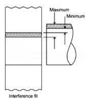
It is used for components where motion, power has to be transmitted.
