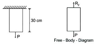
Hence in both the cases reaction at the support will be same which is equal to the load applied on the rod.
